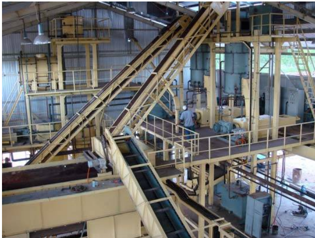
The machinery inside the mill, at the background the pressing platform with 20 tons/hr capacity
