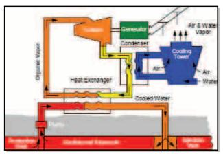
Figure 23: Schematic of a binary cycle (source: Idaho National Laboratory 2011)
