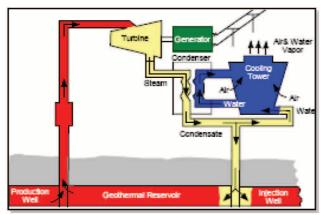
Figure 21: Schematic of a direct steam cycle (source: Idaho National Laboratory 2011)
