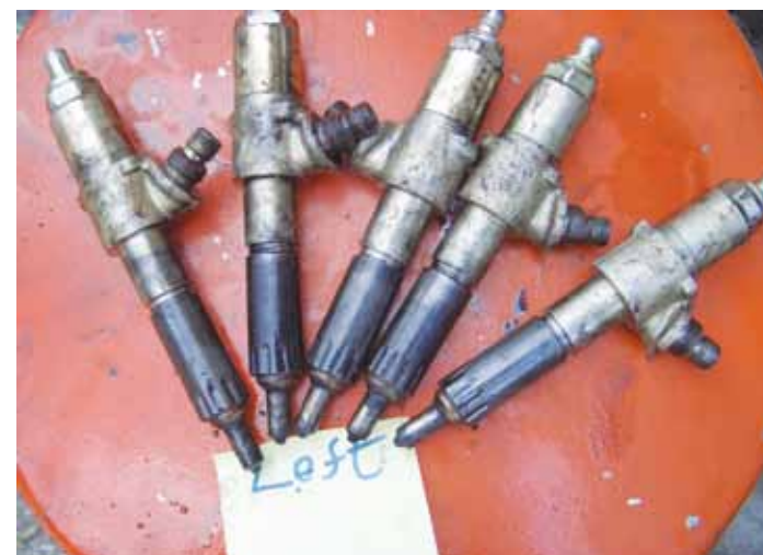
Injection nozzles removed from the engine for inspection. (Photo by NES/LAUDS)
