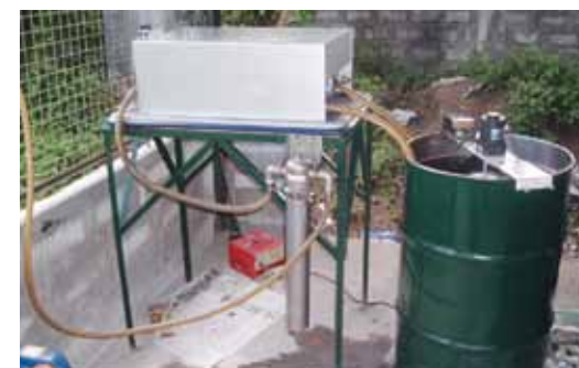
A small MHF machine owned by LAUDS Technologies, Inc. and Nippon Ecosolutions, Ltd. located at the pilot jatropha oil extraction plant owned by Philippine Forest Corporation. Jatropha oil is processed through the reactor (silver-colored, rectangular-shaped machine) and the five-micron tubular filter (silver-colored vertical tube in the middle) while a proprietary additive is added (green drum fitted with a mixer). (Photo by LAUDS Technologies, Inc., 2007).
