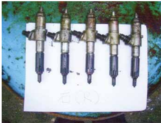
Appearance of fuel injection nozzles removed from the engine of a truck that runs on diesel fuel. (Photo by LAUDS Technologies, Inc. and Nippon Ecosolutions, Ltd.)
