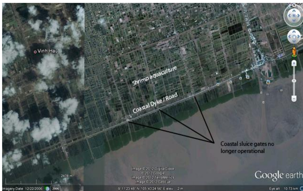
Figure 28. Coastal sluice-gates are no longer operational and left in disrepair in Vinh Hau District, Bac Lieu.
