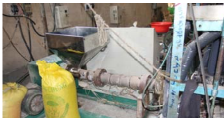
Poor insulation of equipment in a plastic company before CP-RE
