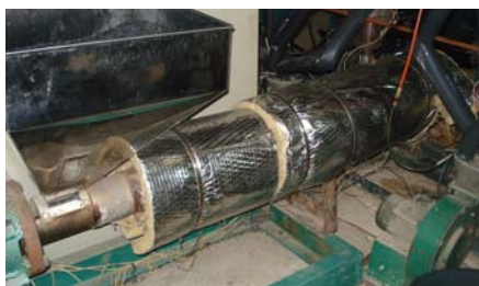
The equipment is now insulated properly
