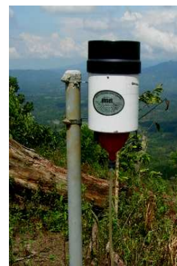
Figure 4. Automatic rainfall measuring device
