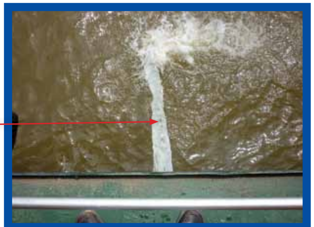
Figure 11: Current Bilge water disposal
