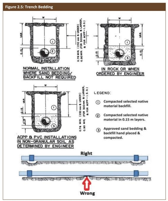
pipe. Bedding is used when the trench bottom does not provide load-bearing capacity suitable for the pipe. The bedding required depends on the pipe material, size and loading over the backfilled trench.
