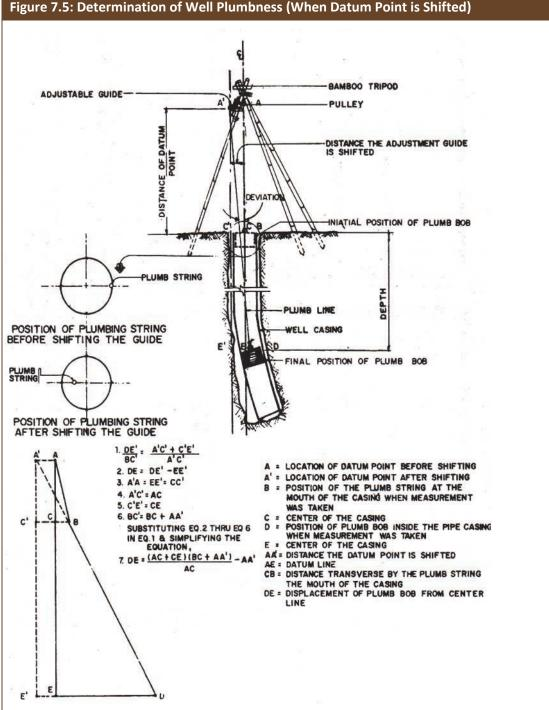
Figure 7.5: Determination of Well Plumbness (When Datum Point is Shifted)
