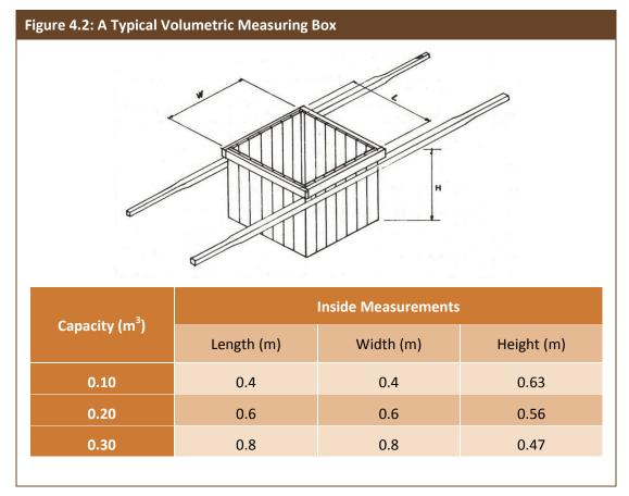
Figure 4.2 shows a typical volumetric measuring box. The inner dimensions should be measured to give the total volume of mix to be prepared at a time.
