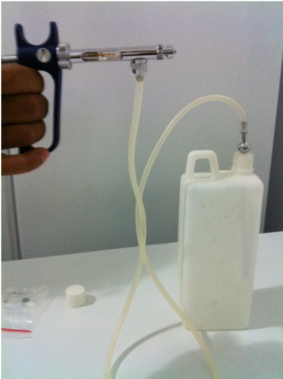
Figure 5. Automatic injection for liquid inoculum.
