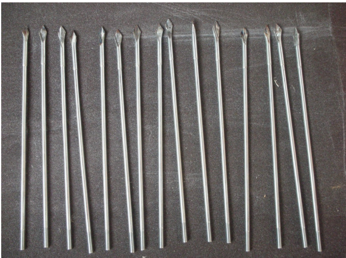
Figure 4. A tool for making an inoculation hole made by radial of motor cyclist.
