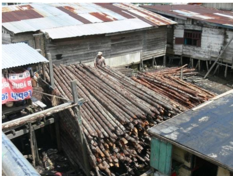
Figure 5. Bruguiera and Rhizophora poles taken from Bulungan mangrove forest, East Kalimantan, for construction works (Photo: Ilman, 2009)
