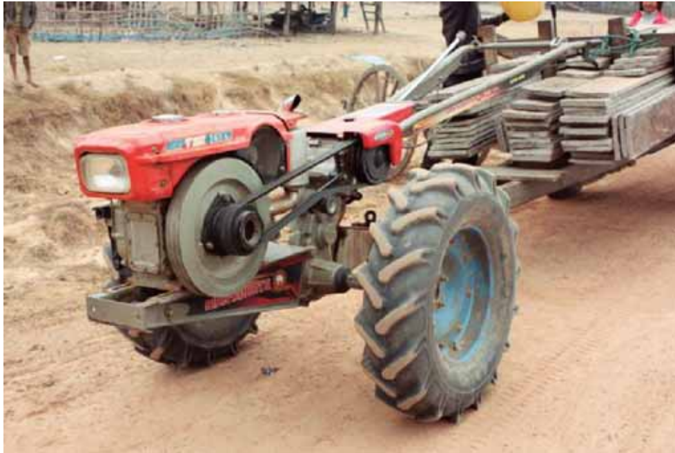
Figure 2 A hand-tractor, here being used to transport construction wood.
