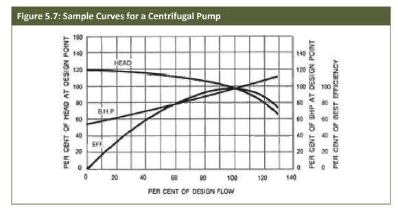
Periodic checking of the pumpset (pump and motor) will disclose deterioration of operation before any serious problems develop. A performance check should be carried out every year or as often as required, especially when the pump is subjected to severe conditions such as corrosion, sand pumping, abrasion or cavitation.
