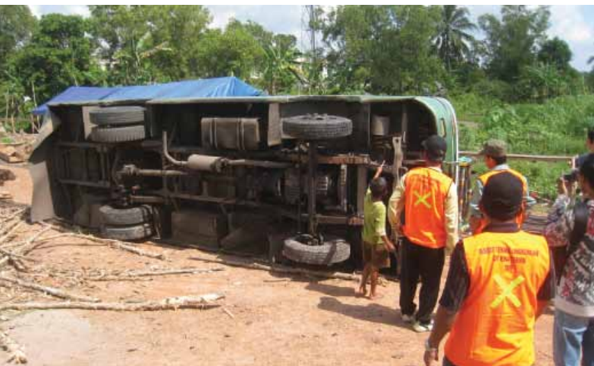
Participants in an IndII workshop on road safety in Palembang came across this bus crash, where an apparent steering failure led to the bus running off the road and rolling over. One person in the bus was killed. Courtesy of Phillip Jordan
