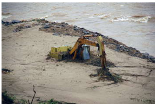
Photo 3.4(Quan Hóa 08/2006). A excavator is buried in muddy when regroup in lower location. It's expensive experience.
