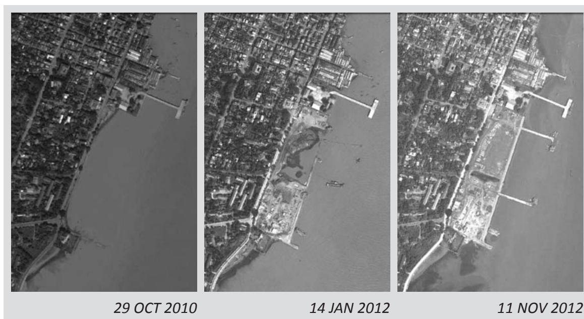
Figure 5 - Satellite imagery showing progress of Site-tway Port land reclamation 29
