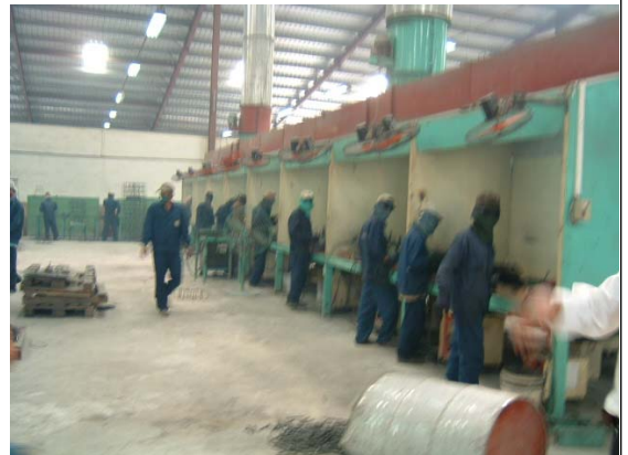
Sep 2006: Welding area with welding booths and air ventilation.
