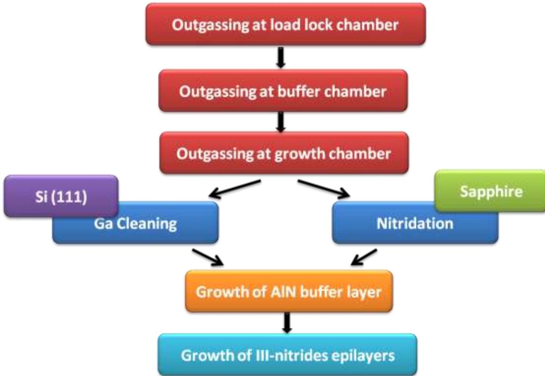
Fig. 3.2 PAMBE growth procedure of III-nitrides thin film on Si (111) and sapphire.
