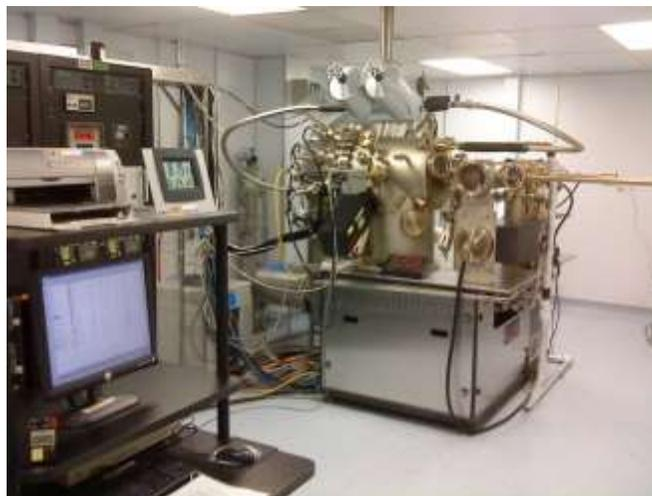
Fig. 3.1 Plasma-assisted molecular beam epitaxy (PAMBE) system.
