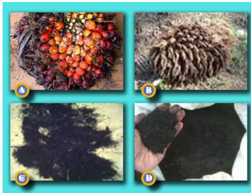
Figure 3: (A) Palm oil fruit bunch; (B) Empty fruit bunch (EFB); (C) EFB biochar; (D) Close-up of biochar [3]
