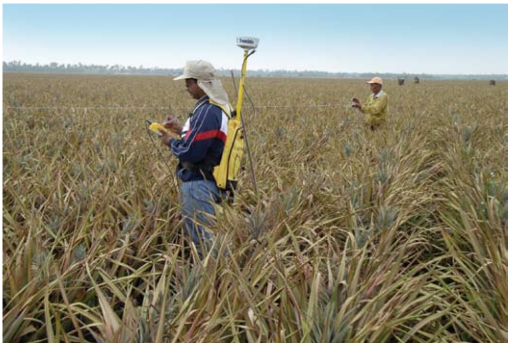
Using a Global Positioning System (GPS) to record location data in a tropical peat land cultivated with pineapple.
