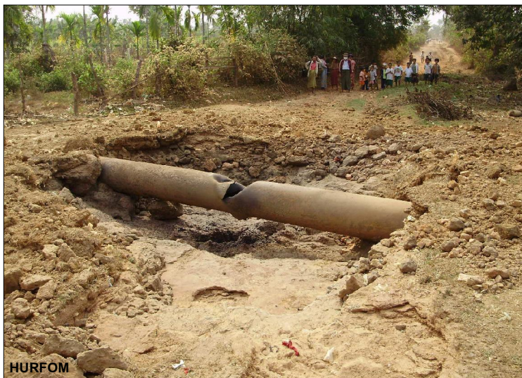
Ruptured pipeline surrounded by a crater left by escaping gas near Lamine Town, northern Ye Township
