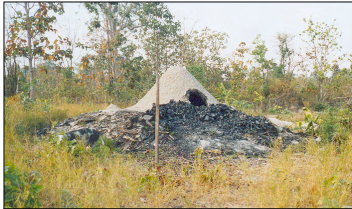
Photograph 5: A charcoal oven used for converting common grade wood, collected in the forest, into charcoal.
