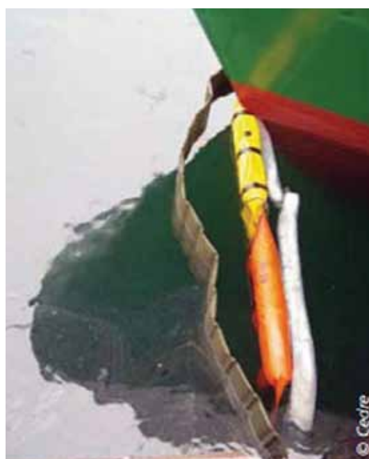
Figure 58: Fence boom (grey), curtain boom with foam filled floats (orange), self-inflating curtain boom (yellow), sorbent boom (white) 38
