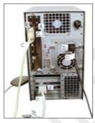
The investigator can place a tag on the video cable labeled "A." Then label the video port on the back of the system also with the letter "A." This way the investigator will know that cable "A" connects to port "A." This method, also known as "Bagging and Tagging," should be done for each cable connected to the system.
