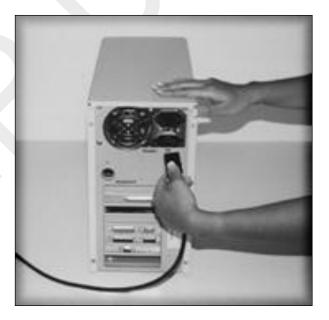
This will make sure the investigator is removing the correct power supply and not another systems power. Shutting down (using the Operating System) will alter the registry and it will be considered as tampering of evidence.
