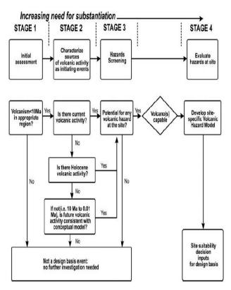
Fig. 14. Methodological approach in determining site suitability of a nuclear power plant site (IAEA 2009). This approach was followed in this study.
