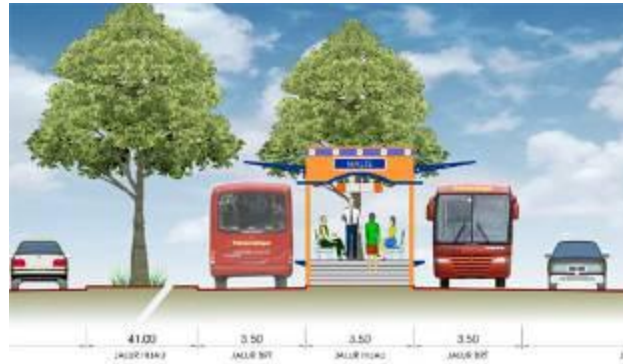
Figure 32: Example of narrow (3.5 m) station design
