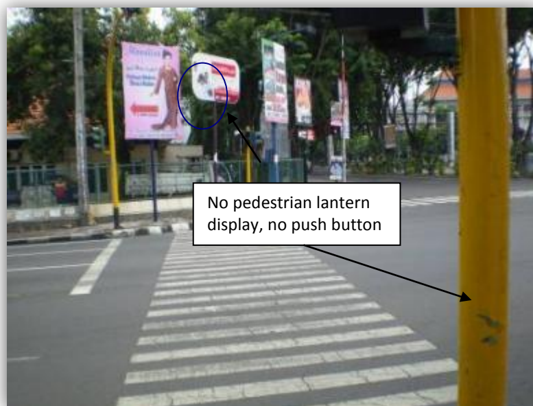
Figure 9: Typical pedestrian crossing where the pedestrian lantern is not operating
