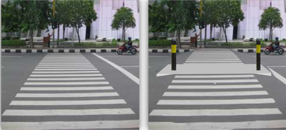
Figure 41: Existing signaled pedestrian crossing and proposed schematic modification to raise the crossing and add a safety refuge
