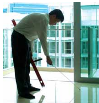
A BCA officer using the CONQUAS Rod to detect hollowness beneath a tiled surface.
