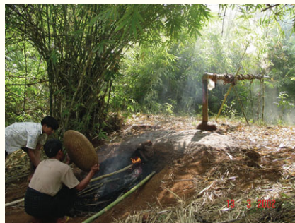
Firing the kiln for making charcoal acid from bamboo for pest control
