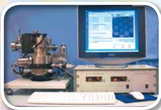
The world's first mobile scanning electron microscope.
