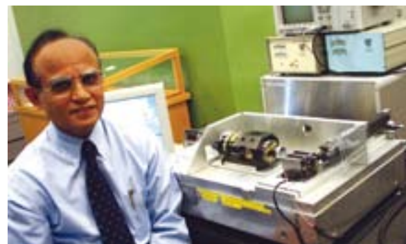
Prof M Rahman with the miniature diamond lathe for nanosurface generation.
