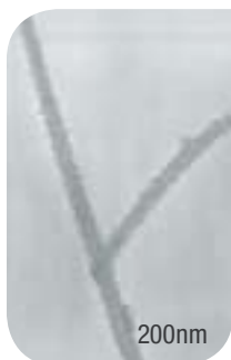
Polyaniline Y-junction nanorod.
