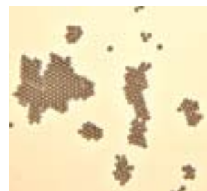
Nucleation of colloidal spheres (polystyrene particles) under an alternating electric field.
