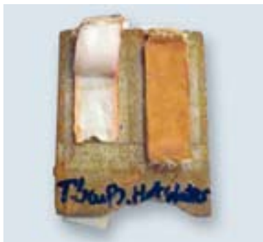
Total cohesive failure is shown in the peel adhesion test of a commercial sealant to concrete after 28-day immersion in 70°C water.
