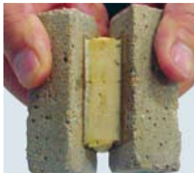
Perfect cohesion and adhesion shown on the heat-resistant polyurethane sealant.
