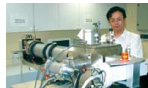
Assoc Prof Liu Xiang Yang working at a small angle X-ray scattering machine that categorises nanostructure.
