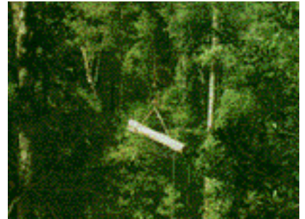
Up, up and away... Timber harvesting using the skyline yarding system
