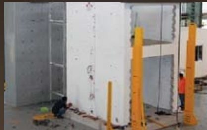
Seismic behaviour of 2 storeys IBS residential under quasistatic lateral cyclic loading
