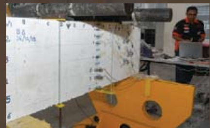
Flexural capacities of high strength reinforced concrete deep beam
