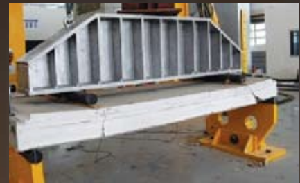
Hollow core slab under shear & flexural test
