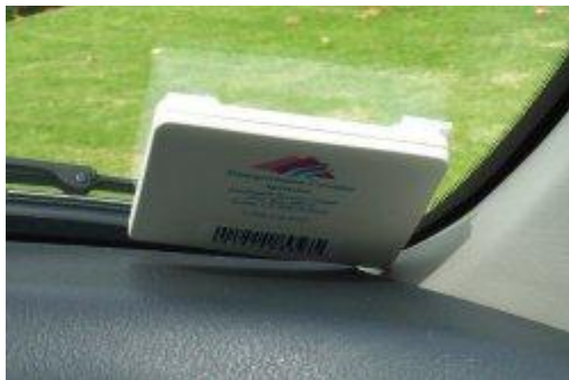
Fig. 1.2.4.1.2. RFID-tag for vehicle identification
