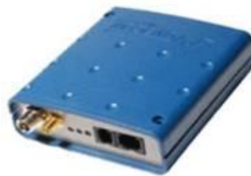
Fig. 1.2.4.3.4. GPS/GLONASS vehicle tracker
