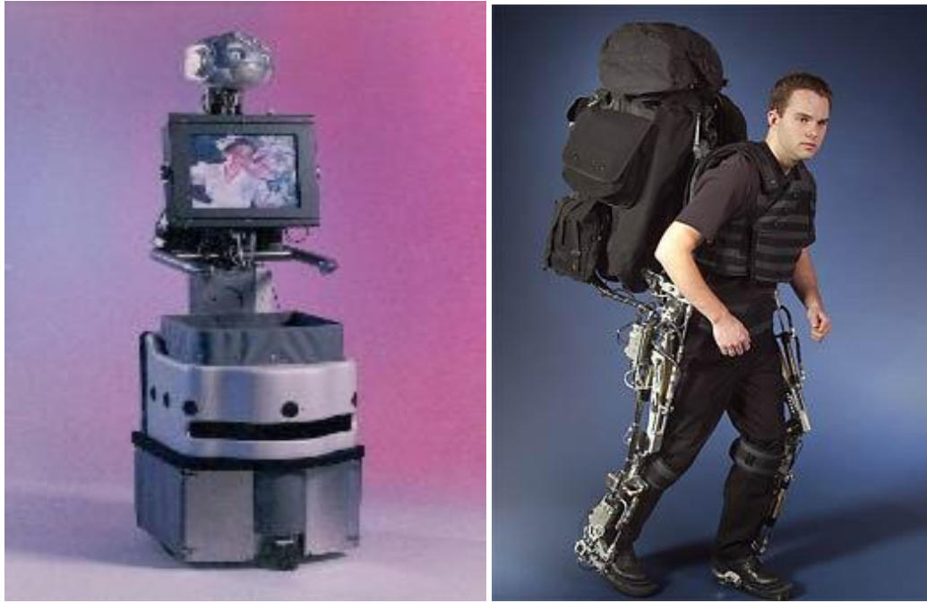
Figure 4: The Nursebot Robot and the Berkeley Lower Extremity Exoskeleton (BLEEX) 99
