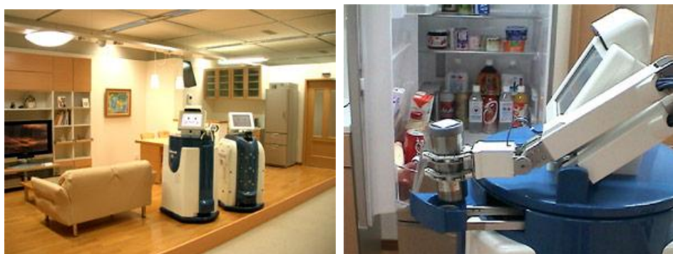
Figure 7: Coordinated operation among a life-supporting robot system (RT space), a refrigerator and a mobile robot 38
