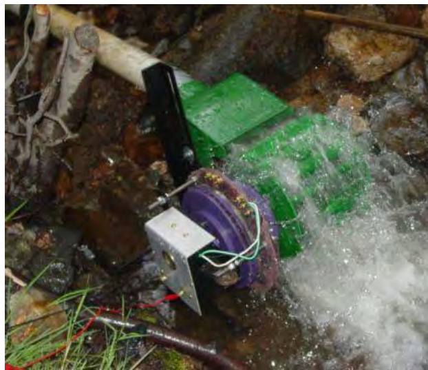
FIGURE 9-21 : Water wheel for micro hydroelectricity power plant
