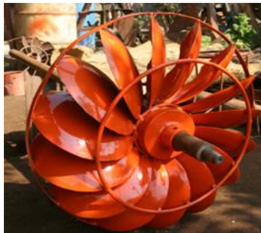
Metal runner for an improved water mill
