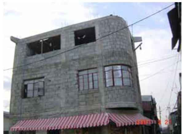
Figure 7. Non-engineered vulnerable construction in Marikina city (relocation site)
